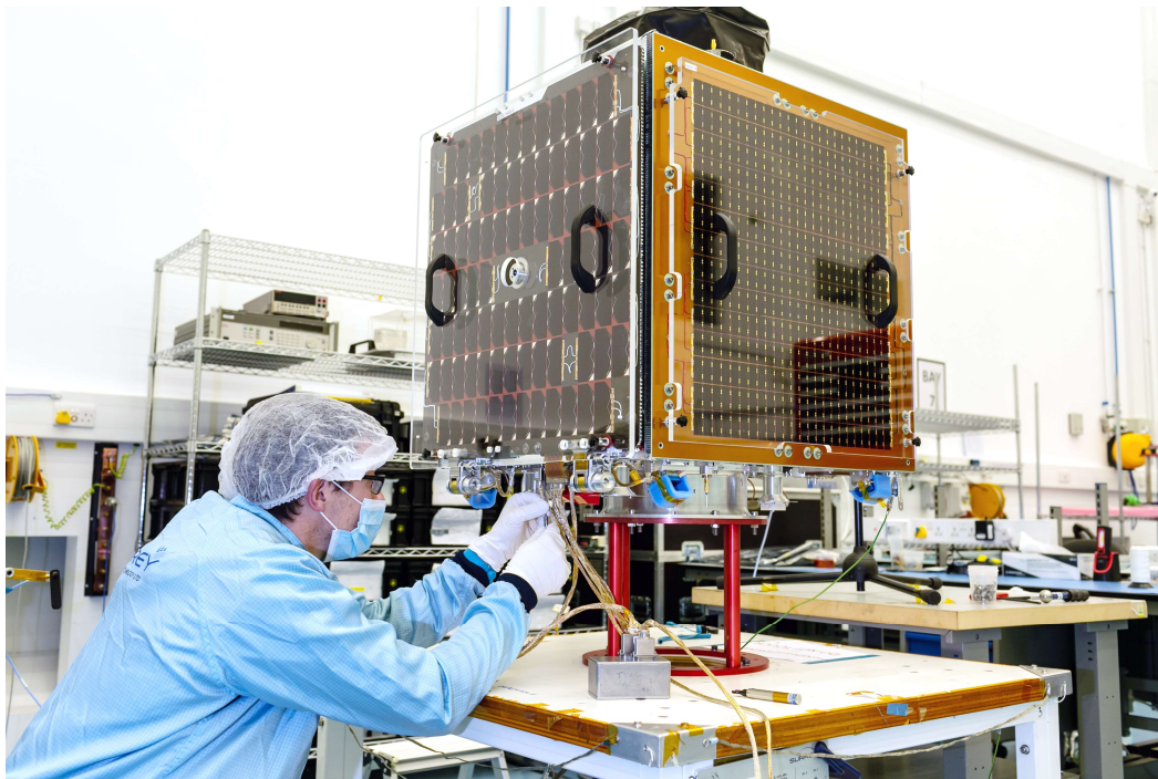
The THEOS-2 SmallSAT during final assembly and testing at SSTL's cleanrooms in the UK. Credit SSTL.
