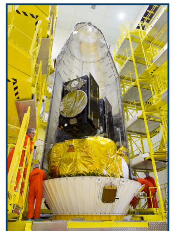
Two Galileo satellites, with solar arrays folded, ready for launch aboard Soyuz
